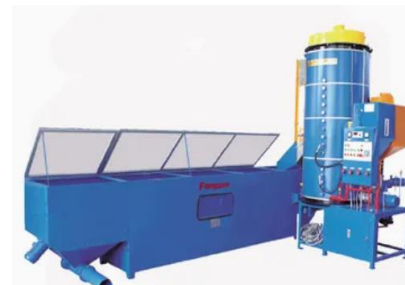
Expansion of plastic particles into Styrofoam particles
